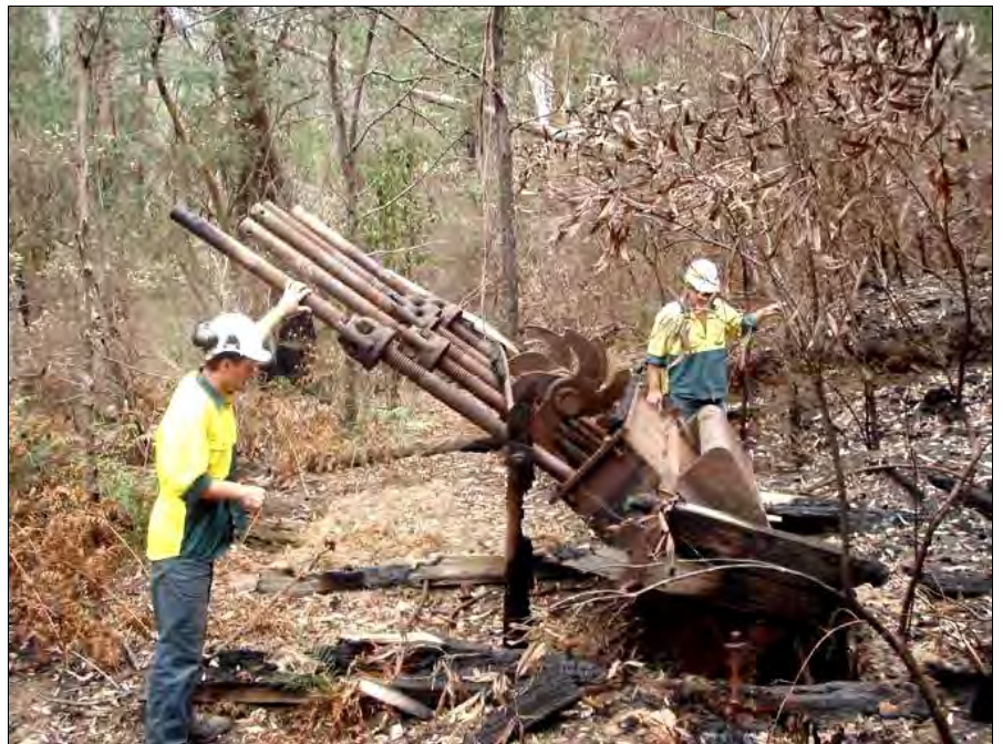
Image at Right: The Langland's Battery in the aftermath of the 2007 Great Divide fire, leaning at a perilous angle, with its wooden frame burned away. Photo: Mal Smith, 2007.
