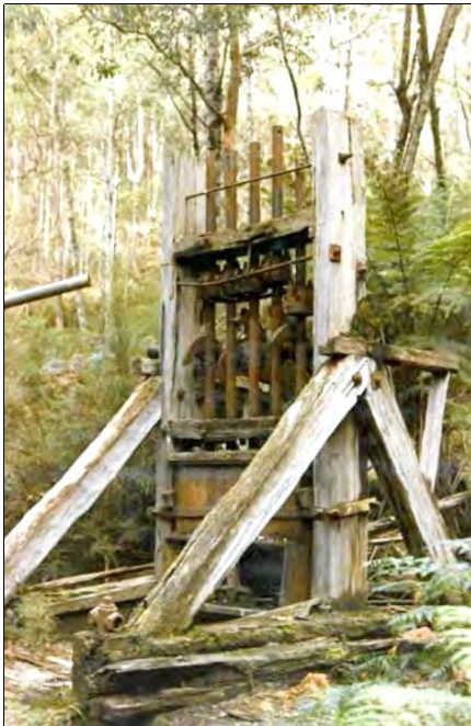
Image at Right: The Langland's Battery in the aftermath of the 2007 Great Divide fire, leaning at a perilous angle, with its wooden frame burned away. Photo: Mal Smith, 2007.
