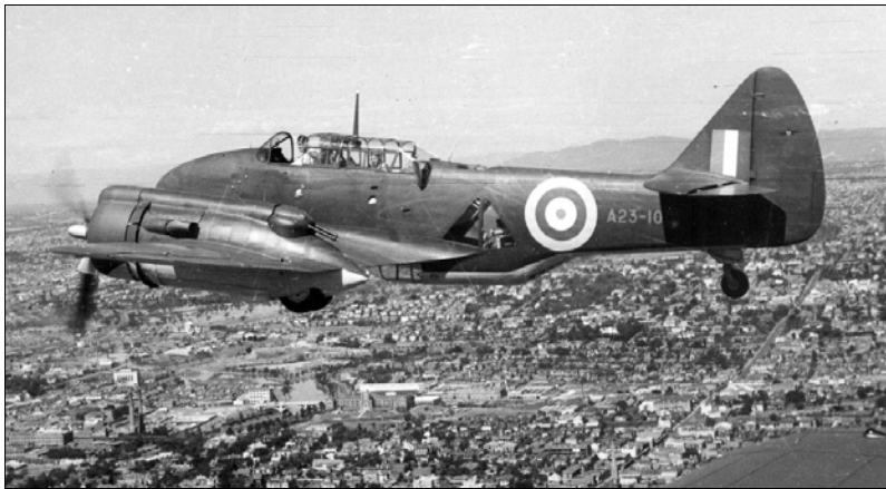
CA-4 Woomera flying over Melbourne - note rear facing gun turrets on the engine nacelles. Source: Commonwealth Aircraft Corporation.
