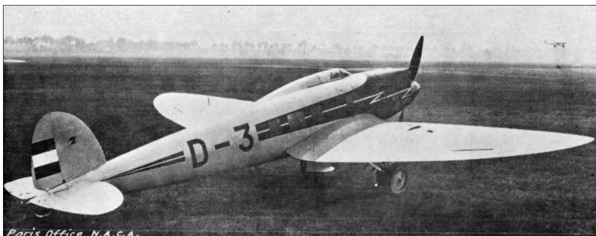
Heinkel HE-70 (Blitz) – elliptical wings and empennage (tail assembly) (1933)
