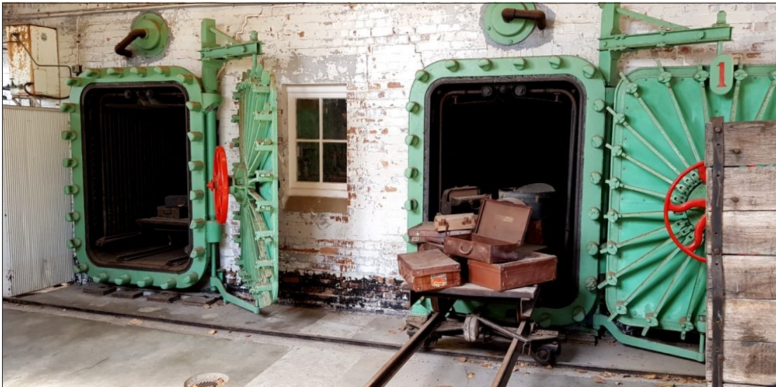
Autoclaves in the Disinfestation Block, in use from 1917 to 1974. Note the movable rails allowing longitudinal and transverse movement of multiple luggage trolleys through either autoclave from where they were parked. Image: Judy Baker.
