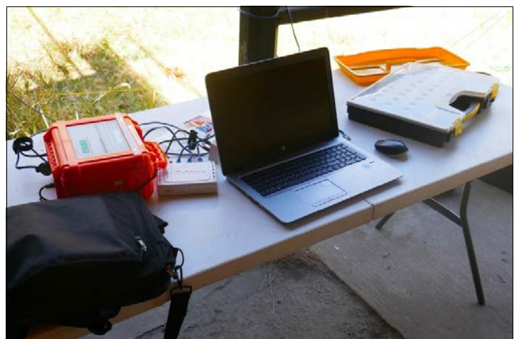
FIGURE 2 : Field setup of a seismic recorder (Networked to a second one).
