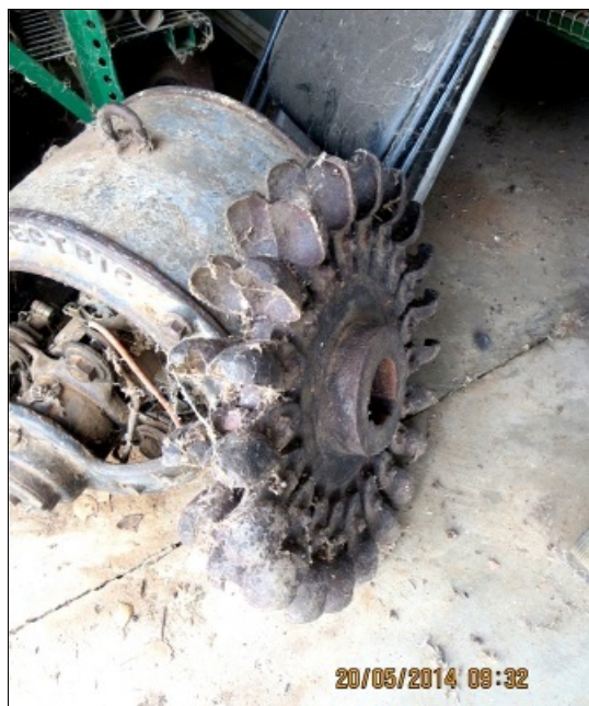
Pelton wheel & WECO generator.
